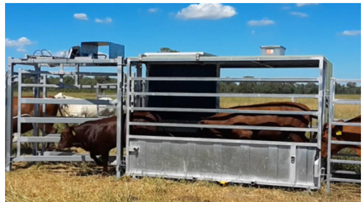
Figure 3. A Walk-over-weigh systems developed by DataMuster™. This systems enables collection of liveweight data on a regular basis while animals are located out in the pasture. This particular system has an “auto-drafter” attached which is being used to sort cows from calves automatically.
