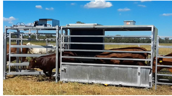
Figure 3 A Walk-over-weigh systems developed by DataMuster™. This system enables collection of liveweight data on a regular basis while animals are located out in the pasture. This particular system has an "auto-drafter" attached which is being used to sort cows from calves automatically.
